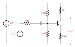
2. In the following circuit, assuming  $\beta \approx 200$  and that  $V_{be} \approx 0.65V$ , find the value of  $R_{b1}$  such that the DC level of  $v_o(t)$  is equal to 8V.
