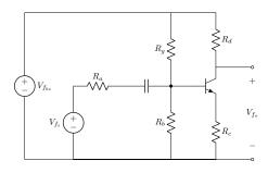
2. In the following circuit, assuming  $\beta \approx Beta$  and that  $V_{be} \approx 0.65V$ , find the value of  $R_g$  such that the DC level of  $V_{f_o}$  is equal to **DC** level.
